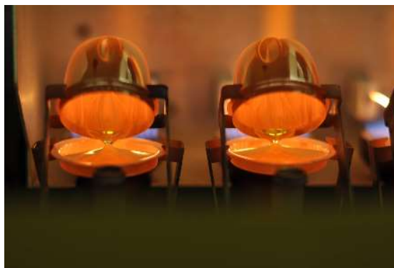
Fused disc manufacture: molten flux and sample mixture poured from the crucible into the disc casting platen.
