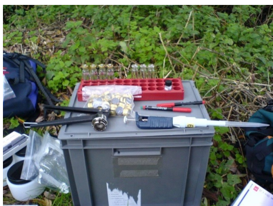
Figure 6: Headspace sampling in the field used for measuring volatile siloxanes.
