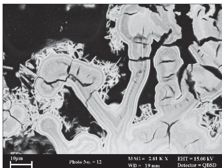
Figure 1 BSEM image showing detail of arsenic-rich iron oxyhydroxide cement coating the surfaces of altered waste fragments. It shows banded colloform oxyhydroxide gel material displaying shrinkage (desiccation) cracks. This is encrusted by more crystalline acicular oxyhydroxide.
