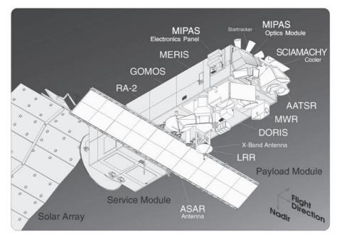
**Envisat** is an advanced Earth observation satellite with a unique combination of sensors to vastly improve the range and accuracy of scientific measurements of the atmosphere, oceans, land surface and ice. Its total range of capabilities far exceeds those of any previous or planned Earth observation satellite. It was launched in spring 2002 by an Ariane-5 launcher.
