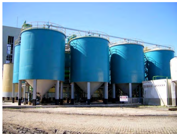
Figure 1: HC Sucroquímica's ABE fermenters (reproduced by permission of HC Sucroquímica)
