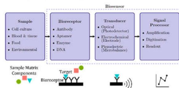
**Figure 1.** Schematic showing the components of a biosensor.
